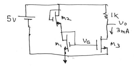
Since Vo = 2V, want VG < 2V+VrH to maintain saturation of M3. So will set VG = 2V  $I_{D3} = \mu (o_{k} \omega) (2 - .75)$  $3E-3 = (E-4) - (1.25)^{2}$  $\frac{1}{L_3} = 38$ . Let  $L_3 = lm$ ,  $w_3 = 38m$ Let  $W_i = 38$  so unity minnor gain Let  $L_i = 1$ ,  $W_i = 38$ , W $I_{01} = 3mA$ Consider now M2. which also has ID = 3mA  $3mA = M for W_2 \left( 5 - V_G - V_{TH} \right)^2$ 3 = (E-4) = (5-2-.15)Solving
