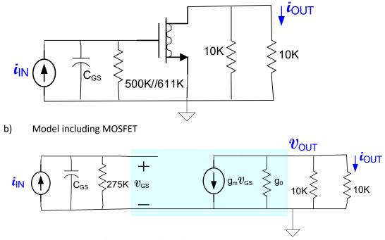
Defining  $R_B=275K$ ,  $G_B=1/R_B$ , and  $G_L=1/R_L=1/10K$  and summing currents at input and output nodes obtain equations
